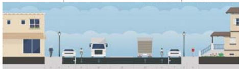
Section A (G Street to E Street) 3 Lanes - Remove Travel Lanes, Add Bike Lanes, Add Street Lighting
